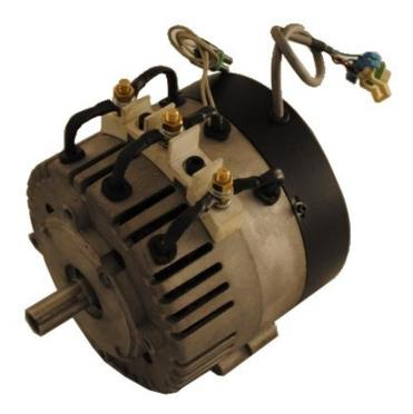
Manufacturer description: Output Power of 12 KW Continuous, 30 KW Peak (at 96 volts)
